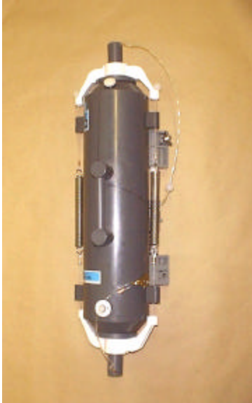
5-liter Niskin-X bottle without 3-thermometer reversing assembly.
